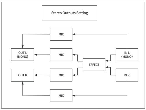
For the IN L&R, the dry signal and wet signal sounds are mixed when OUT L&R.
