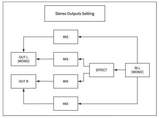
• For the **IN L**, the dry and the wet sounds are mixed when stereo output.
