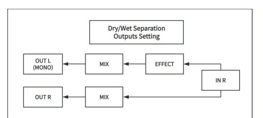
• Dry/Wet Separation output : For the IN R, OUT R carries the dry signal; OUT L carries the wet signal.
